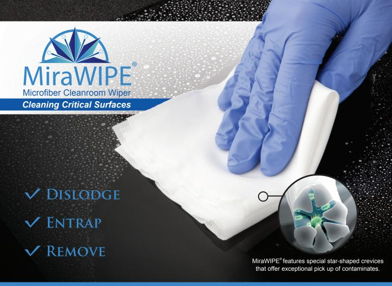
MiraWIPE® is a sealed edge microfiber wiper constructed from continuous filament micro denier nylon/polyester yarn to enhance contamination entrapment and removal on critical surfaces. The weave and sealed edge are designed to resist shedding and tearing to prevent in-use particle and fiber severation. Cleanroom washed and packed, MiraWIPE® is available in configurations to meet Class 1-1000 applications.
