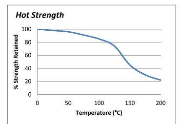
"Hot strength" shear strength tests performed on mild steel. Fully cured then conditioned to pull temperature for 30 minutes before testing. ES569 can withstand higher temperatures for brief periods (such as for paint baking and wave soldering processes) providing the joint is not unduly stressed. The minimum temperature the cured adhesive can be exposed to is -40°C (-40°F) depending on the materials being bonded.
