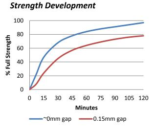
Graph shows typical strength development of bonded components at 23°C. An increase of 8°C in temperature will halve the cure time. Lower temperatures will result in a slower cure time.
