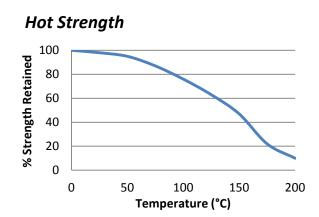
"Hot strength" shear strength tests performed on mild steel. Fully cured specimens conditioned to pull temperature for 30 minutes before testing at temperature. TA439 can withstand higher temperatures for brief periods (such as for paint baking and wave soldering processes) providing the joint is not unduly stressed. The minimum temperature the cured adhesive can be exposed to is -55°C (-65°F) depending on the materials being bonded.
