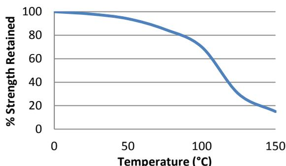
"Hot strength" shear strength tests performed on mild steel. Fully cured specimens conditioned to pull temperature for 30 minutes before testing at temperature. TA435 can withstand higher temperatures for brief periods (such as for paint baking and wave soldering processes) providing the joint is not unduly stressed. The minimum temperature the cured adhesive can be exposed to is -55°C (-65°F) depending on the materials being bonded.
