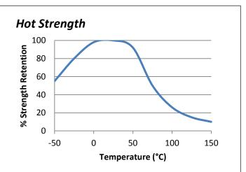
"Hot strength" shear strength tests performed on mild steel. 24hr cure at room temperature and conditioned to pull temperature for 30 minutes before testing.
