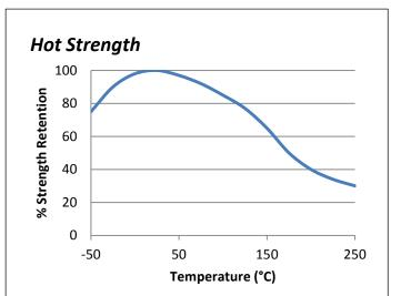
"Hot strength" shear strength tests performed on mild steel. Initially cured at room temperature and then post-cured at 150°C for 2 hours. Test pieces conditioned to pull temperature for 30 minutes before testing.
