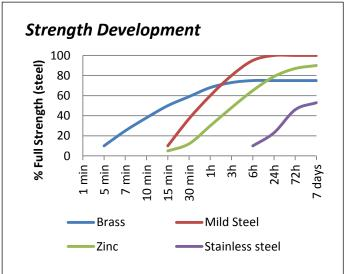
\*Cure times are typical at 23°C. Copper and its alloys will follow the faster cure while oxidised or passivated surfaces like stainless steel will tend towards the slower curve. Lower temperatures or large gaps will tend to extend the cure time. To reduce the cure time the use of Permabond A905, ASC10, or heat can be considered.
