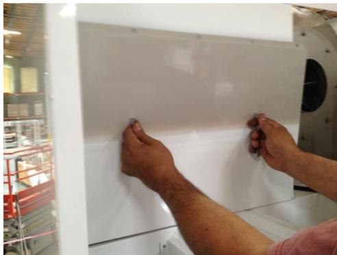
**Photo 28:** Inside panel door shown being removed
