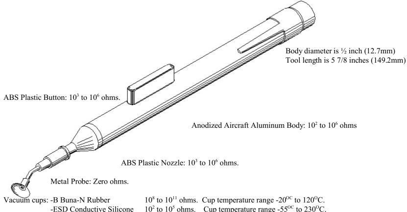
NOTE: The maximum handle to tip resistance is determined by the highest resistance item of the tool in question. Example: If you are using the tool with the -B Buna-N rubber vacuum cups then the handle to tip resistance will be 10<sup>8</sup> to 10<sup>11</sup> ohms.
