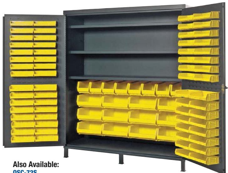
QSC-72S-84 NEW 72"W x 24"D x 84"H. Flush Door model. Ship wt. 955 lbs. Total of 84 bins. 32 QUS232, 32 QUS236, 8 QUS240, 12 QUS250 and 3 adjustable shelves. 500 lb. capacity per interior shelf.
