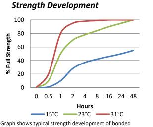
components. An increase of 8°C in temperature will halve the cure time. Lower temperatures will result in a slower cure time.
