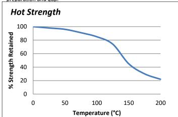
"Hot strength" shear strength tests performed on mild steel. Fully cured then conditioned to pull temperature for 30 minutes before testing. ES569 can withstand higher temperatures for brief periods (such as for paint baking and wave soldering processes) providing the joint is not unduly stressed. The minimum temperature the cured adhesive can be exposed to is -40°C (-40°F) depending on the materials being bonded.
