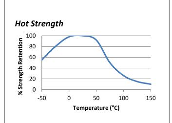
"Hot strenath" shear strenath tests performed on mild steel. 24hr cure at room temperature and conditioned to pull temperature for 30 minutes before testina.
