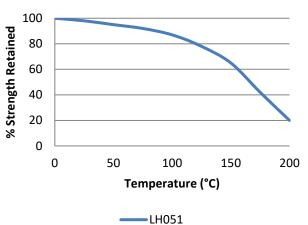
"Hot strength" Breakaway strength on M10 Zinc plated bolts according to ISO 10964. Cured at 23°C for 24 hours then conditioned for 30 minutes at testina temperature.
