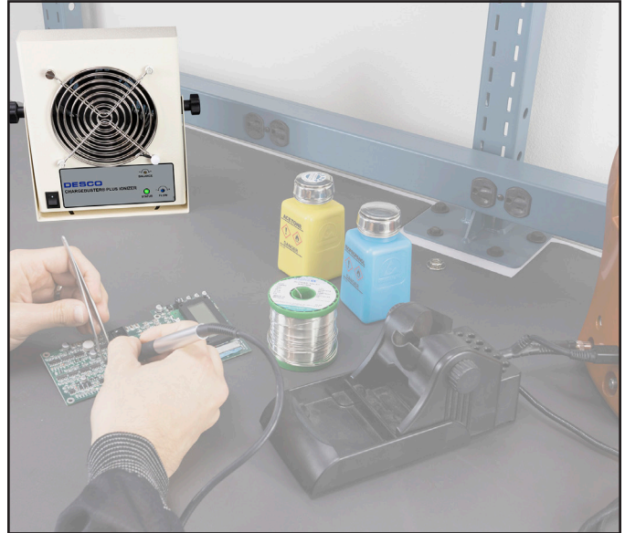
Figure 6. Using the Chargebuster Plus Single-fan Ionizer on a workbench
