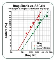
**Durafuse® LT** samples in the chart (left) experienced a peak reflow temperature of 210°C and demonstrated drop shock resilience similar to that of SAC305.
