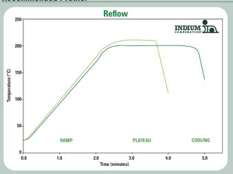
This profile is designed for use with **Durafuse® LT** (Indium10.8HF). This can be used as a general guideline in establishing a reflow profile for **Durafuse® LT** Solder Paste. Deviations from these recommendations are acceptable, and may be necessary, based on specific process requirements.
