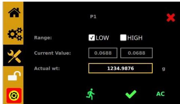
Figure 12: Advanced Calibration Screen (LOW)
