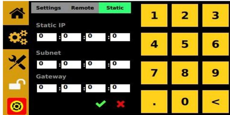
Figure 39: Setting a static IP address
