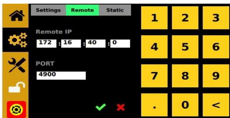
Figure 38: Setting the IP address and port
