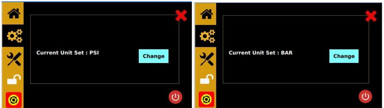
Figure 17: Press “Change” to change the pressure units
