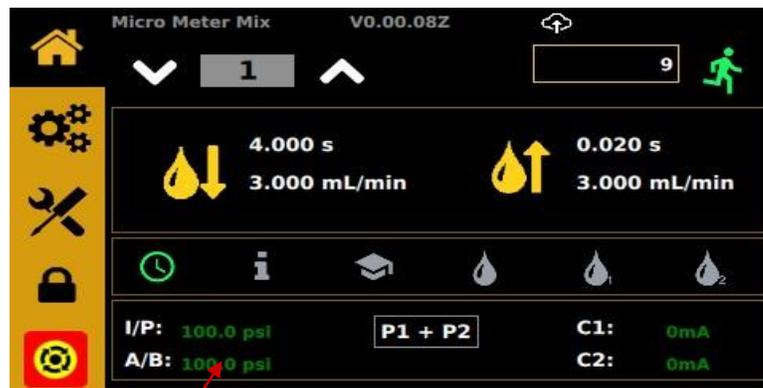
Figure 15: Output Pressure Display
