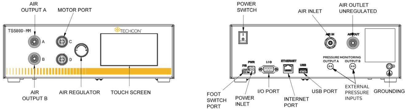
Figure 1: Controller Features
