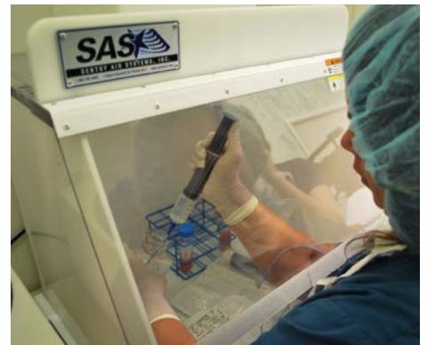
The 18" PCR Hood provides a sterile workspace for a variety of medical applications
