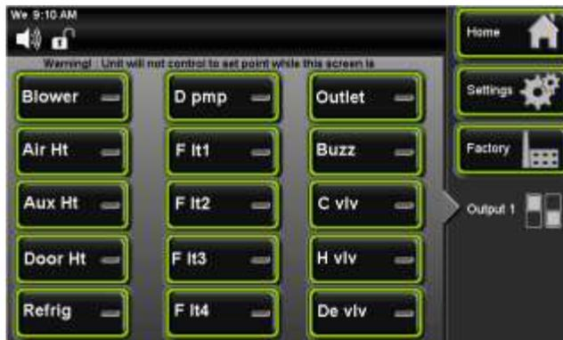
Each item can be turned on to check the condition of that device or parameter to aid in diagnosing a problem.
