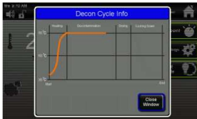
The Decon Cycle Info Screen will appear displaying the current stage that the Decon Cycle is in.
