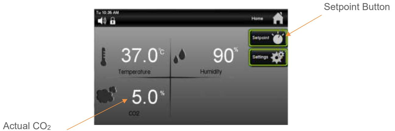
To set the CO<sub>2</sub> setpoint, press the
