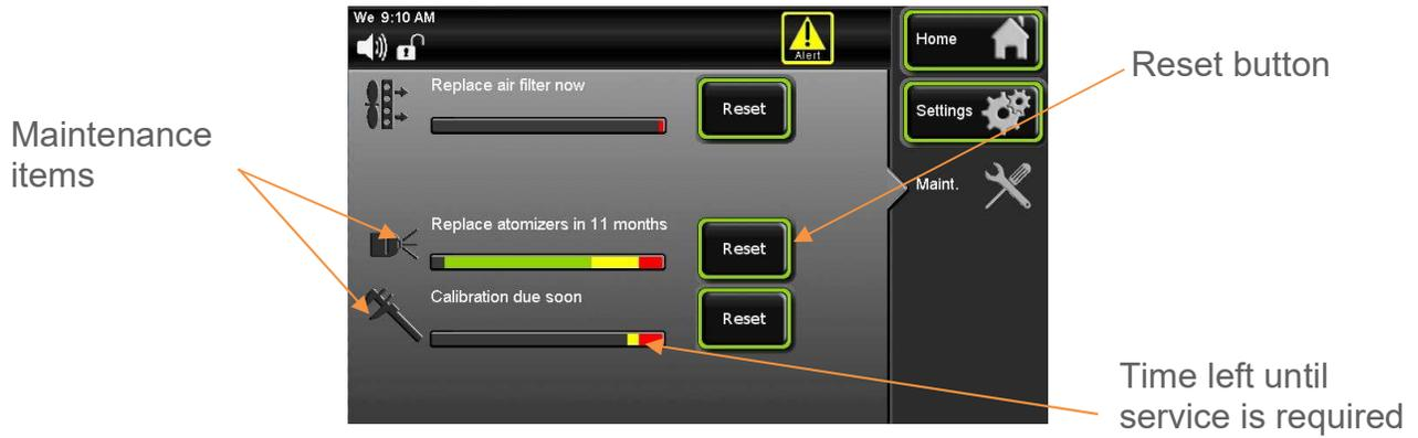
Once a Maintenance item is displayed on the Alert screen, it will continue to be present as an icon in the Status Bar until the Maintenance item is corrected and the (Reset) button is pressed resetting the replacement time to “new” status.
