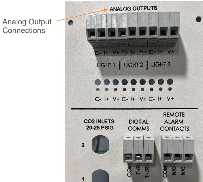
Analog outputs provide either a milliamp (4-20mA) or voltage (0-5V) signal output to represent each of the displayed temperature, humidity or CO<sub>2</sub> values. These options can be used for connection to in-house data acquisition, recorder, or alarm system. The temperature parameter (only) is adjustable in its scaling and is accessible at the Analog Output screen.
