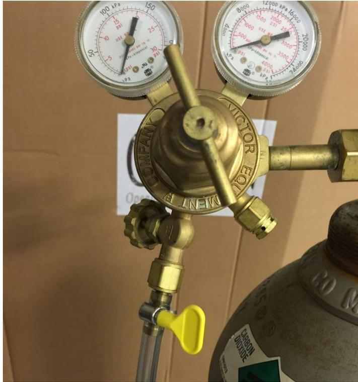
The CO<sub>2</sub> supply should be 99.5% and not have siphon tubes. CO<sub>2</sub> pressure should be regulated to 15-20 psi. CO<sub>2</sub> tank regulators can be purchased through CARON customer service. Once the cylinder regulator is installed, connect the outlet of the regulator to the hose barb fitting using the tubing and clamps provided.
