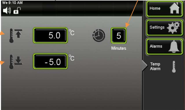
The screenshot shows a control panel interface. At the top, it says 'We 9:10 AM'. On the left, there are two vertical sliders for temperature limits. The top slider is labeled '5.0 °C' and the bottom slider is labeled '-5.0 °C'. To the right of these sliders is a clock icon and a box labeled '5 Minutes'. On the right side of the screen, there is a navigation menu with buttons for 'Home', 'Settings', 'Alarms', and 'Temp Alarm'. The 'Temp Alarm' button is highlighted with a red box.
