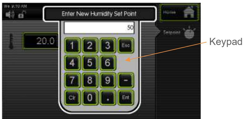
Enter the new humidity setpoint on the keypad as desired and press
