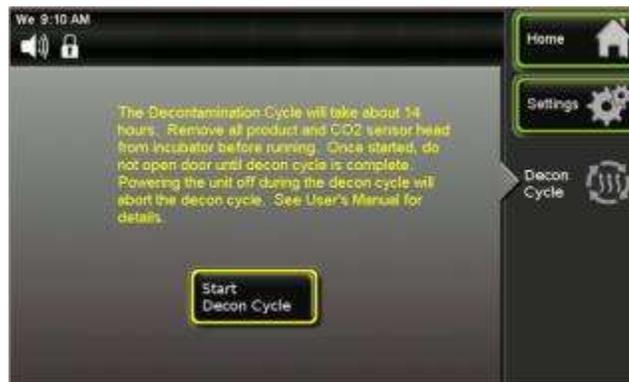
Be sure and read the information that is on the screen before starting the Decon Cycle. Not removing the sensor can cause damage to the CO<sub>2</sub> sensor.
