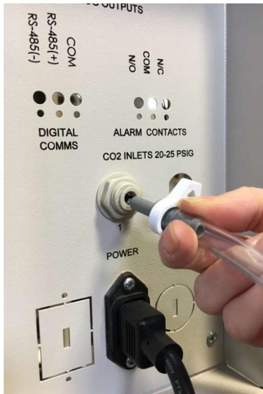
An inline HEPA filter is provided to remove any contaminants in the CO<sub>2</sub> gas supply. Check the connections closely for leaks.
