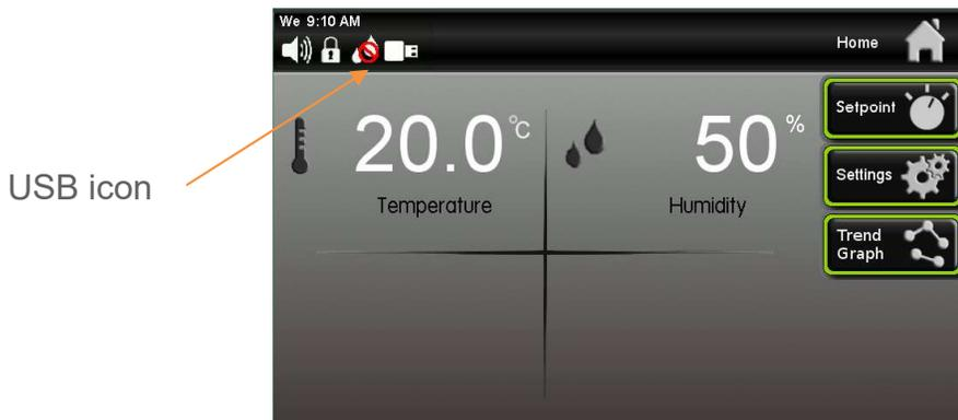
USB icon appears in in Status bar indicating that data is being written to flash drive. To retrieve the data press the 'Eject' button, then insert the flash drive into a computer to upload the data.
