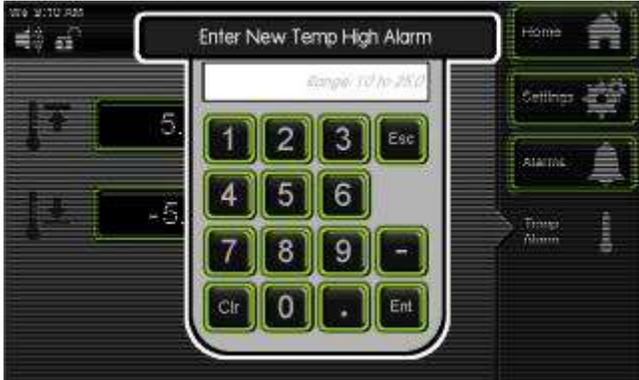
The screenshot shows a keypad interface. At the top, it says 'Enter New Temp High Alarm'. Below this is a text input field with the value '5.0' and a label 'Range: 10 to 25.0'. The keypad has buttons for numbers 1-9, 0, a decimal point, and function keys like 'Esc', 'Ent', and 'Clr'. On the right side, there is a navigation menu with buttons for 'Home', 'Settings', 'Alarms', and 'Temp Alarm'. The 'Alarms' button is highlighted with a red box.
