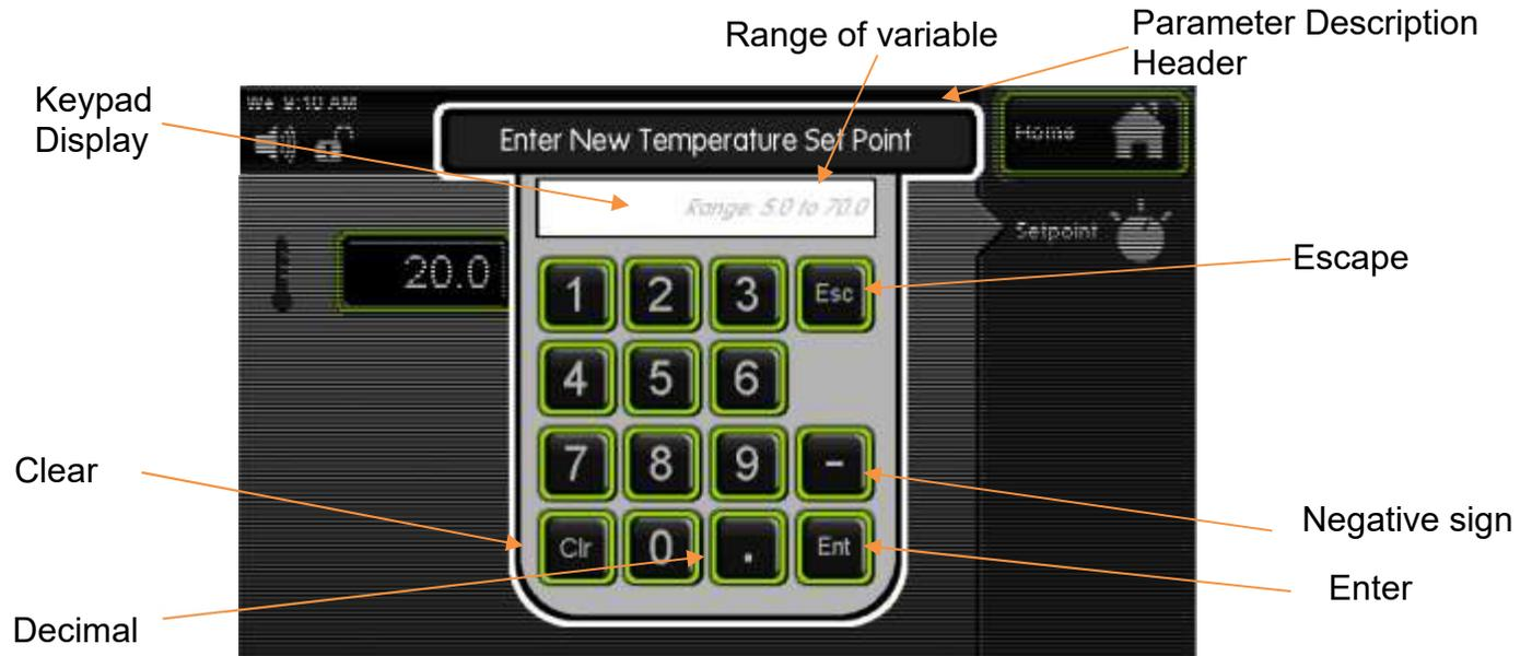
The Parameter Description Header tells what parameter is being changed. The Keypad Display shows allowable values of the parameter being changed (initially) and displays the entered value (when a button is pressed).
