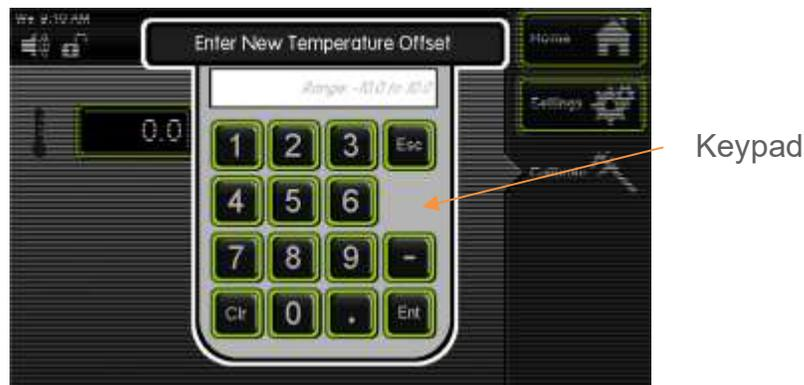
Enter the temperature offset by using the keypad and pressing
