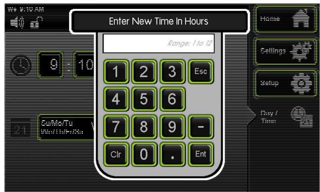
The Enter New Time in Hours window will appear. Enter the hour by using the keypad
