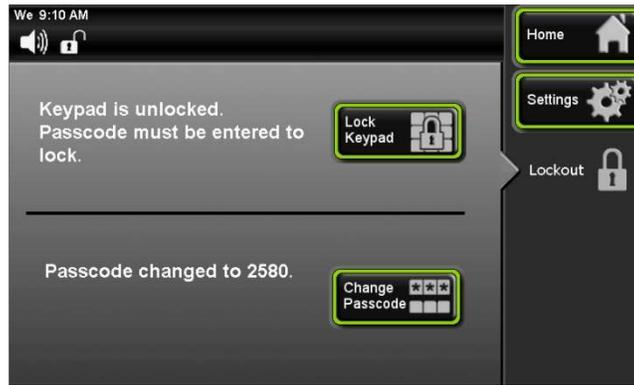
The Lockout screen will tell you that the Passcode has been changed to a new value. *This is only time that the Passcode will be displayed on the Lockout screen.*
