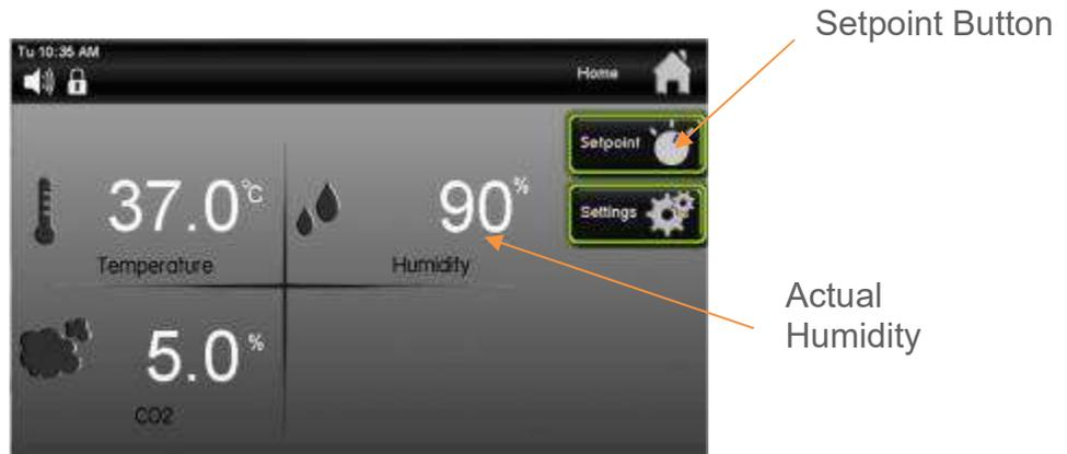
To set the humidity setpoint, press the
