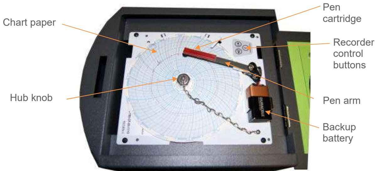
Press and hold the “change chart” button on the recorder (#3) for approximately one second until the pen begins to move to the left of the chart and then release the button. Wait until the pen has completely moved off of the chart. To remove the chart paper,
