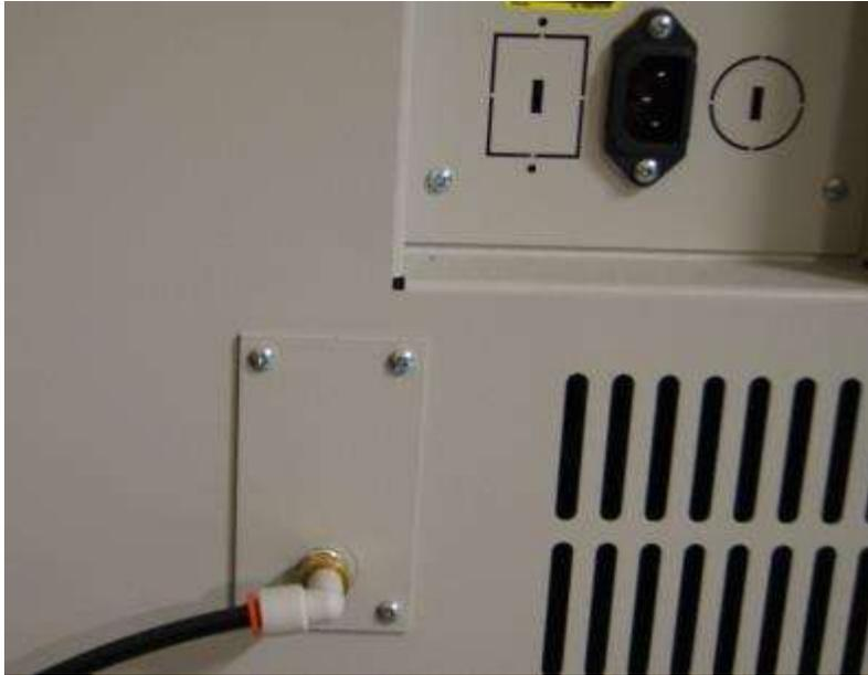
A water inlet fitting on the back of the unit and 1/4" black tubing are provided to connect the water supply to the incubator. Connect an appropriate water supply to the fitting. Incoming line pressure should be regulated to not exceed 80 psi.
