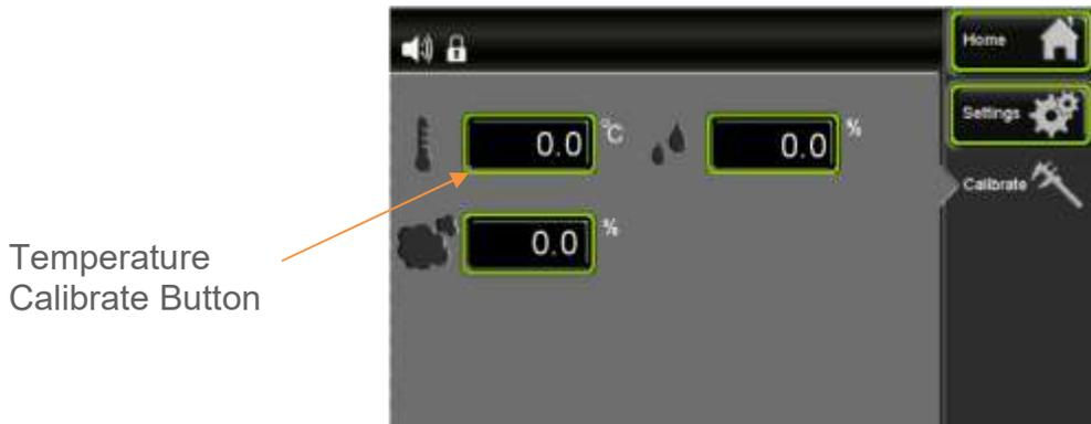
At the calibrate screen, press the
