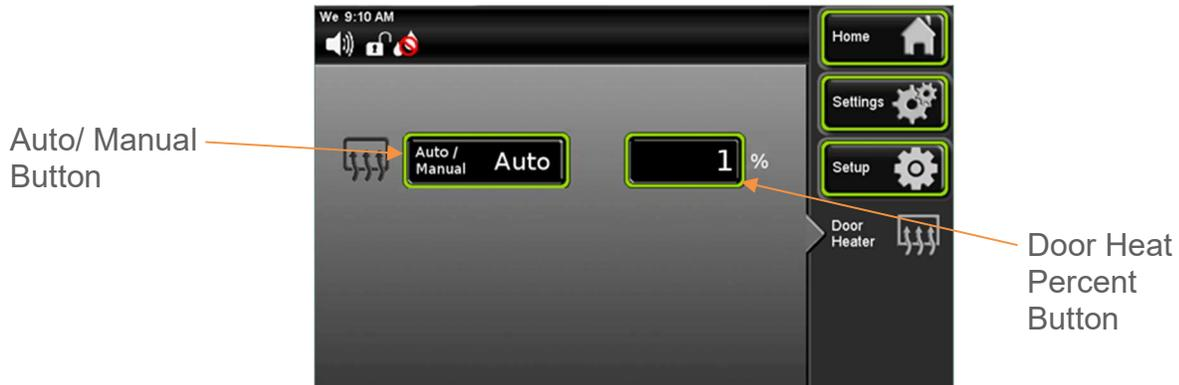
In Automatic mode, the door heater works in conjunction with the internal heaters to maintain the temperature set point. In the event that the temperature is above set point, the door heater will automatically throttle back.
