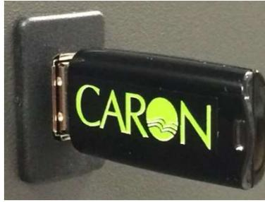
The DLOG301 option provides the customer with a means of logging data electronically for viewing at a later date. Logged variables are Temperature, Humidity, CO<sub>2</sub> and Light Intensity (but only if the chamber is equipped with those features.) All data is time-stamped with year, month, day of the month, hour, minute, 24 hour time (ISO 8601 format). This data is stored internally in the chamber in non-volatile memory.
