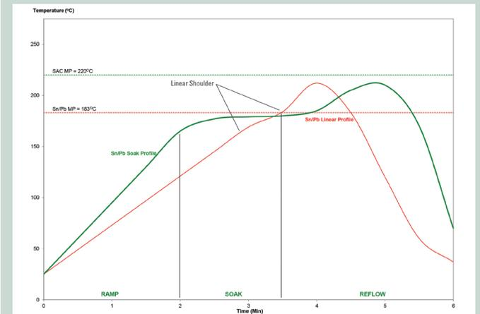
The stated profile applies to Sn63 and Sn62 alloys. This can be used as a general guideline in establishing a reflow profile when using NC-SMQ®92H solder paste. Deviations from these recommendations are acceptable, and may be necessary, based on specific process requirements, including board size, thickness, and density. Start with the linear profile, then move to the optional soak profile if needed. The flat soak portion of the linear profile (linear shoulder) may also be eliminated.
