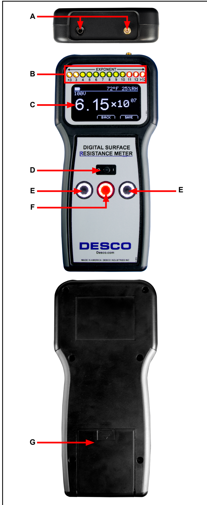
Figure 4. Digital Surface Resistance Meter features and components
