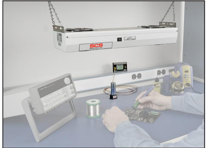
Figure 22. Using the EM Aware Monitor with ionizer antenna on a workbench with the SCS [770112 Ion Pro™](#) Overhead Ionizer
