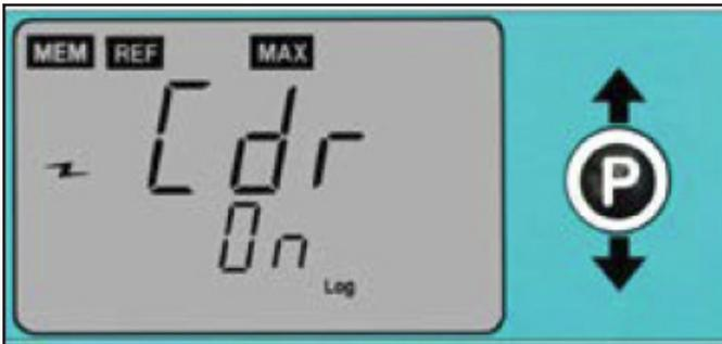
Figure 12. Enabling the noise filter
