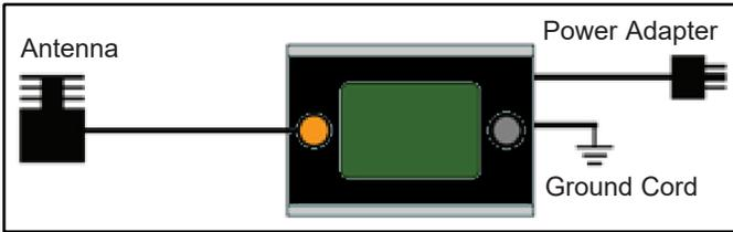
Figure 6. Stand-alone setup for the EM Aware Monitor
