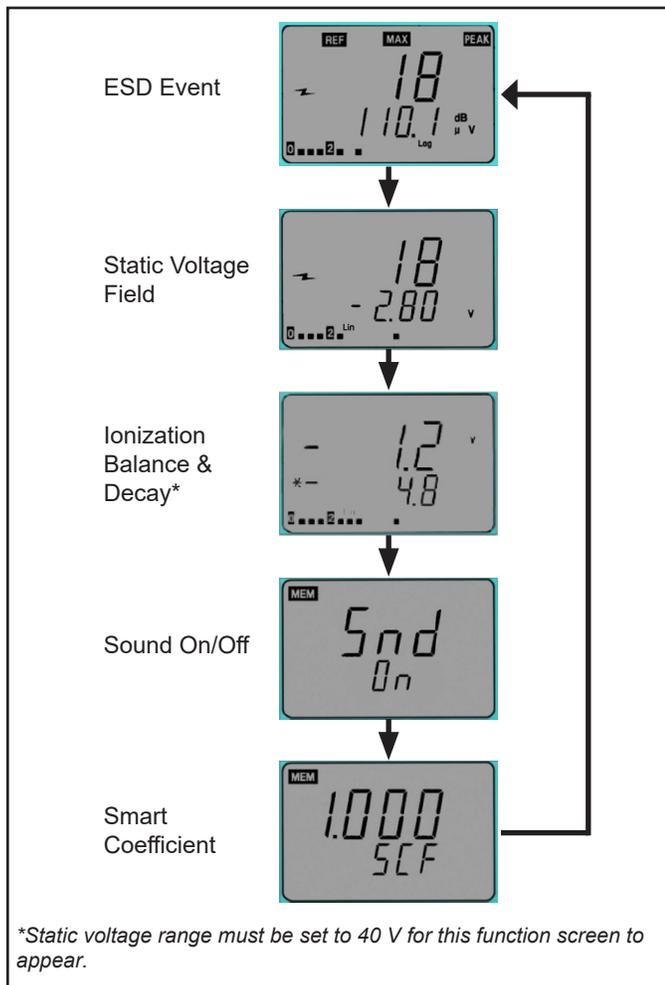
Figure 9. Cycling through the modes on the display
