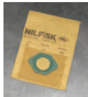
The electrostatic paper bag offers finer filtration capabilities, retaining 97.8% of particles down to 1.5 microns. Its electrostatically charged inner lining is comprised of meltblown polypropylene to attract ultra-fine particles, enabling the bag to capture materials such as toner. *(Continued on next page)*
