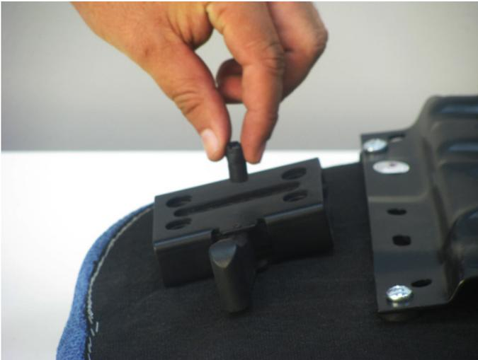
1. Remove the end travel retention pins. Slide out the arm lock cam handle.
