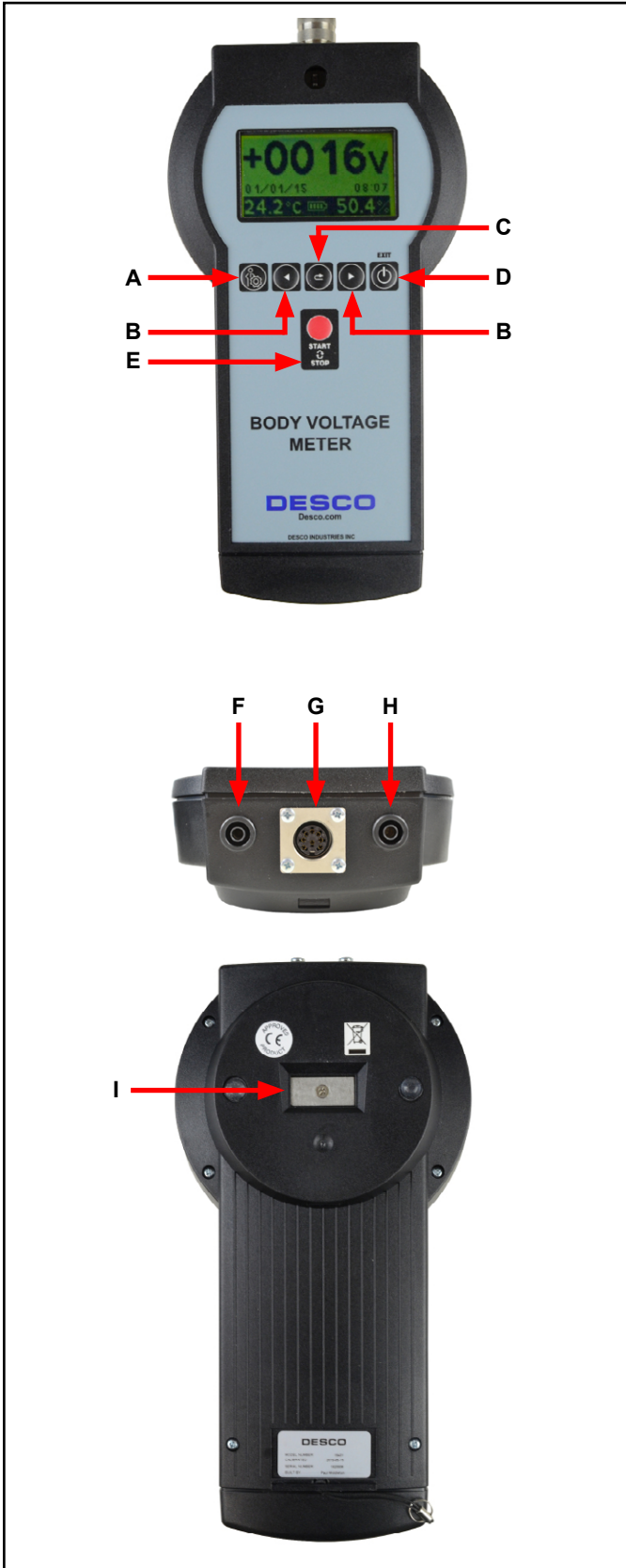
Figure 2. Body Voltage Meter features and components
