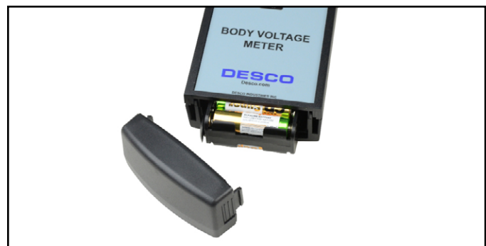
Figure 7. Replacing the Batteries on the Body Voltage Meter
