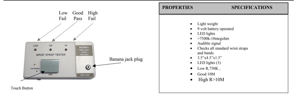
Insert 9v battery into compartment and plug banana jack from wrist strap into back from banana hole and push down on touch plate. To test just coil cords, unplug coil cord from strap, plug banana end into jack in back of unit with snap end in hand touch coil head to touch plate pressing down. If unit you are testing is good green LED will come on.
